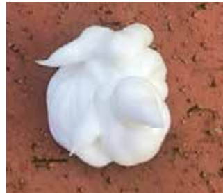
KÖSTER Crisin Cream is firm. This is an advantage when working from cartridges and tubular bags. Even when too much product is applied into the borehole, excess material will not run down onto the plaster that can lead to dark spots afterwards. Excess material can be removed and the borehole subsequently filled and plastered over.
