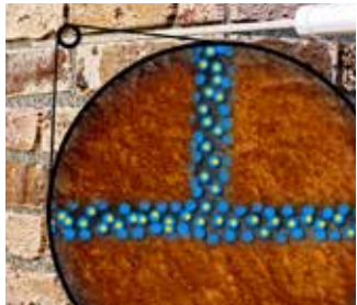
Conventional creams: The product mixes with pore water. In the case of damp masonry the active ingredient is diluted, lowering its concentration and the distribution of the active ingredients in the masonry is uncontrolled.
