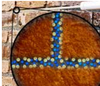
KÖSTER Crisin Cream: No mixing of the active ingredients with water due to the reversed formulation. On the contrary, water is bit by bit displaced, the active ingredients remain in the desired position.
