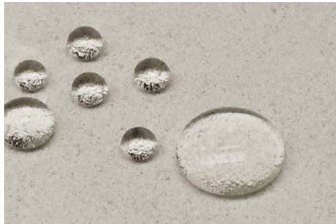
Hydrophobizing: Making the building material water repellent
