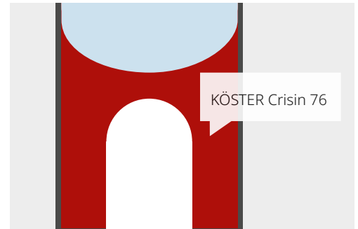
Narrowing/blocking the capillary, forming an elastic film in the capillary/reduce the pore diameter
